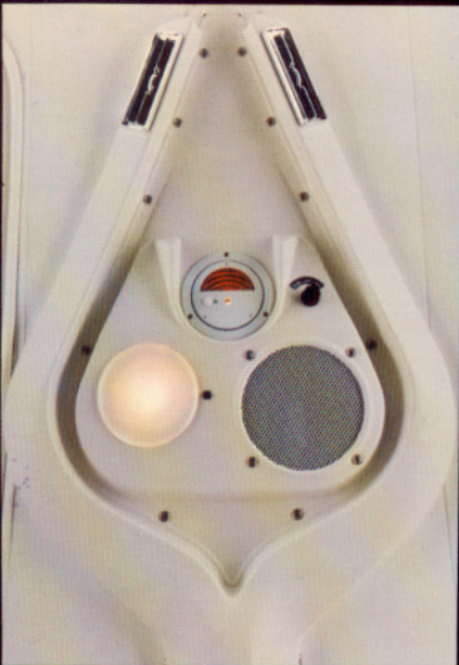
A ram air ventilation system and combustion heater help maintain a comfortable in-flight cabin environment.
